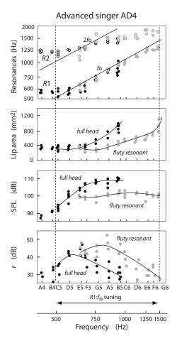
FIG. 7. Comparison of vocal tract resonances R1 and R2, lip articulation, sound pressure level (SPL,) and the difference r in harmonic level [defined by Eq. (1)] between "full head" (black symbols) and "fluty resonant" (gray symbols) productions by advanced singer AD4. See caption to Fig. 4 for further details.
