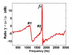
FIG. 10. (Color online) The measured pressure ratio  $\gamma$  for the note A6 (~1750 Hz) sung by the non-expert singer NE1. The second vocal tract resonance R2 is adjusted to the first voice harmonic  $f_0$ .
