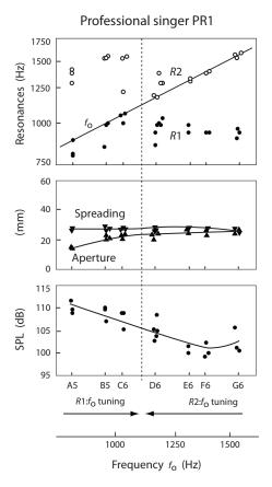
FIG. 12. The variation of vocal tract resonances R1 and R2, lip opening area and sound pressure level (SPL) with increasing pitch for the professional singer PR1 over the range A5 to G6. The vertical dashed lines across the three panels indicate the ranges of  $R1:f_0$  and  $R2:f_0$  tuning for this singer. See caption of Fig. 4 for further details.
