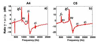
FIG. 9. (Color online) Comparison of the measured pressure ratio  $\gamma$  for the production of the pitches A4 (a) and C5 (b) by the professional singer PR3. On A4 (440 Hz), the first resonance R1 is adjusted to the second voice harmonic ( $2f_0$ ). On C5 (about 500 Hz), the frequencies of R1 and R2 are lowered considerably so they are close to  $f_0$  and  $2f_0$ , respectively.
