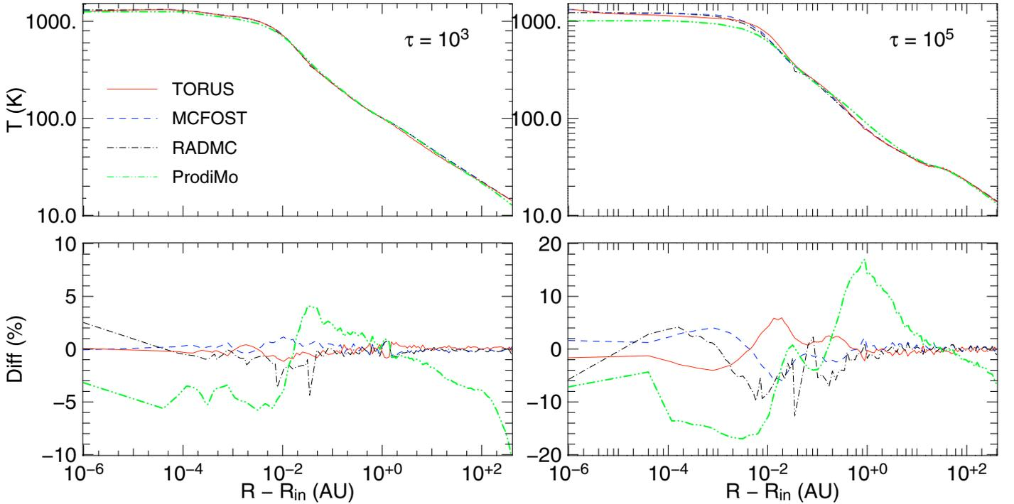
**Fig. 9.** Radial temperature profile in the disc midplane (isotropic scattering). The *left panel* corresponds to the  $\tau = 10^3$  case and the *right panel* to the  $\tau = 10^5$  case. The full red lines represent the results of TORUS, the blue dashed lines, the results of MCFOST, the black dot-dashed lines the results of RADMC and the green dot-dot-dashed line the results of ProDiMo. Differences are relative to the average results of the Monte Carlo codes MCFOST, RADMC and TORUS.
