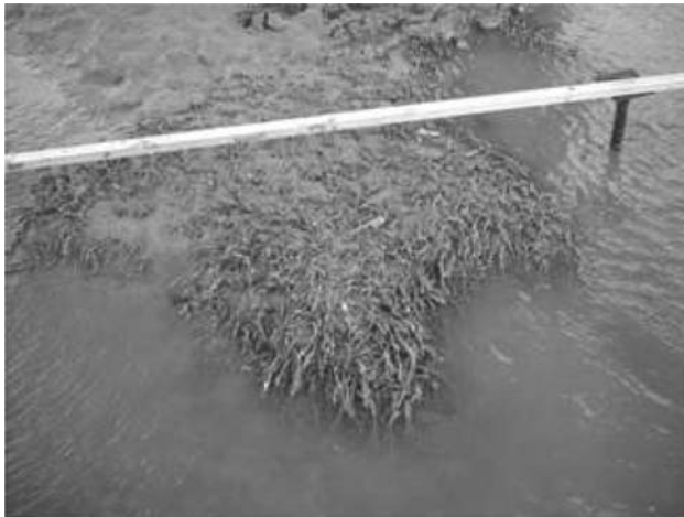
Fig. 3 Methodology to determine the relative height differences of individual aggregations: the vertical distance to the horizontal conduit was measured every 10 cm
