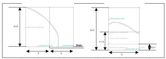
Figure 4: Dams: toe drain and impermeable sheet on the downstream face.
