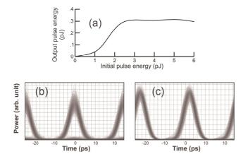
Fig. 7: (a) TF obtained for a bidirectional use. (b) Optical eye diagram at the regenerator input (b) and output (c)  $% \left( \begin{array}{c} c \\ c \\ c \\ c \\ \end{array} \right)$
