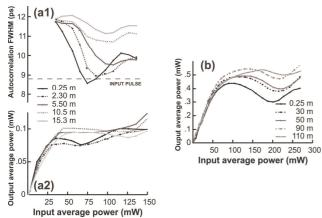
Fig. 9: Influence of the DCF length for different input powers: (a) Results for the 6.4 ps pulse train: output autocorrelation FWHM (a1) and TFs (a2), (b) TFs for the 10 GHz setting for  $\sim$ 20 ps-pulse train.
