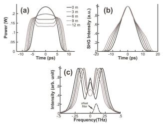
Fig. 5: Influence of the intermediate DCF length on the temporal (a) and spectral (c) intensity profiles obtained before spectral filtering. Fig. (b) is the intensity autocorrelation associated with the temporal profiles of Fig. 5(a).
