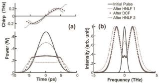
Fig. 3: Numerical evolution of (a) the temporal intensity (bottom) and chirp (top) profiles and (b) of the optical spectrum for an initial pulse energy of 4.5 pJ at various points within the 3-segment configuration.
