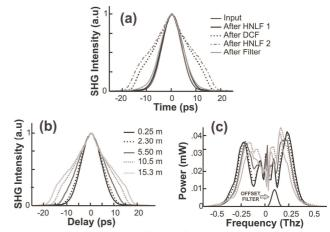
Fig. 8: Experimental results with a 10 GHz, 6.4 ps input pulse train: (a) Autocorrelation traces recorded at different output positions for a 10.5 mlong DCF. (b-c) Influence of the DCF length for an input average power of 110 mW: (b) autocorrelation traces after the DCF before optical filtering and (c) optical associated spectra.
