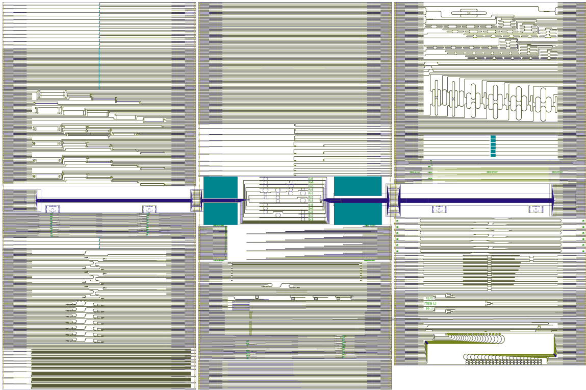
Fig. 2. Mask layout for the 2009-10 course, consisting of a full IMEC FXT cell with a total area of > 12.1 \times 7.4 mm. Twenty-three (23) student designs were merged on this layout. We used IMEC's "fxt3 FC 630" template taking advantage of their predefined vertical fibre coupler shallow etch mask; hence, the students designed only the deep etch mask (a second chip was provided for those who needed to design both the shallow and deep etch masks). This template contains 3 columns of input/output grating couplers, with a coupler pitch of 25 \mu\text{m} . Each column is approximately 4 mm wide, and there is a total of 940 input/output pairs on the chip, of which more than 800 have been used by the student designs.
