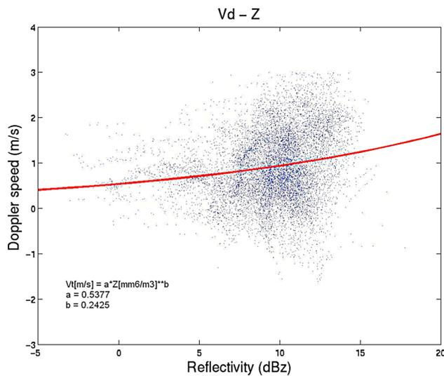
**Figure 18.** Scatterplot of Nadir Doppler velocity versus radar reflectivity measured by the RASTA 95 GHz Doppler radar for all the Falcon 20 flights during AMMA SOP3. The nonlinear regression to these data points is shown as a red line, and the  $a$  and  $b$  parameters are also given.
