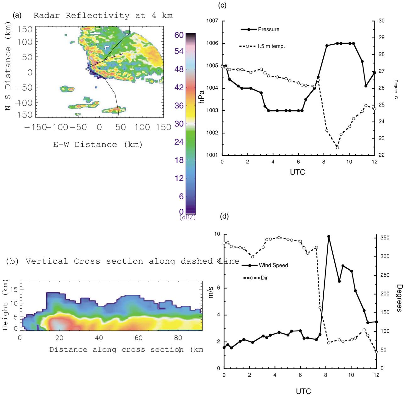
**Figure 8.** 31 August Kawsara measurements of (a) 0800 UTC NPOL Radar 4 km reflectivity, (b) NPOL cross section of reflectivity (dBz), (c) flux tower 1.5 m pressure and temperature, and (d) 12 m wind speeds and direction.
