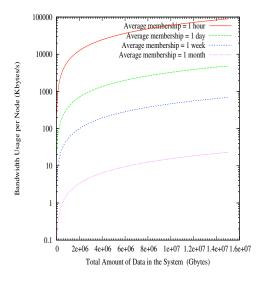
Figure 4: This graph shows the required bandwidth per node function of the churn for maintaining up to 1000 TBytes of unique data at an availability at least equal to 0.99
