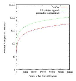
Figure 3: This graph shows the number of stored fragments per node in DataCube, in a full replication approach, and pure rateless erasure coding one. The replication factor used for the full replication approach is equal to 33 (see Figure 2) while the stretch factor for pure coding is equal to 10.
