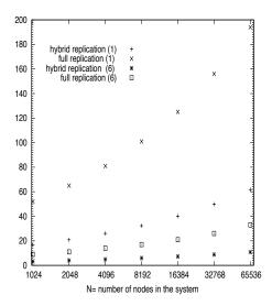
Figure 2: This graph shows the required stretch factor for our solution (hybrid redundancy) and replication factor for the full replication approach in function of N the number of nodes in the system. The required availability is  $d_a = 0.99$ . The number shown in brackets (i.e., 1 and 6) represents the number of redundant routes.
