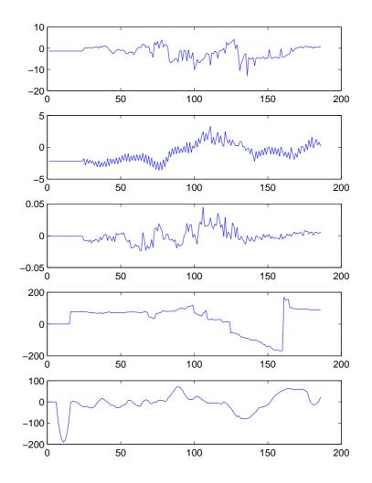
Figure 8: Features observed on the video sequence and used to compute beliefs of Fig. 9. From top to bottom: horizontal motion ( $P_{\rm hm}$ , in pixels by image), vertical motion ( $P_{\rm vm}$ , in pixel by image), zoom ( $P_{\rm div}$ ), angle ( $P_{\rm swing}$ , in degree) and vertical variation of center of gravity ( $P_{\rm vcg}$ , in pixel by image).
