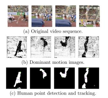
Figure 2: Original video sequence (a), dominant motion images (b) and human point detection and tracking results (c) for a *high jump* (with *running, jumping, falling* and *standing-up* actions).
