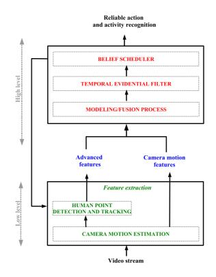
Figure 1: System architecture for human motion analysis.
