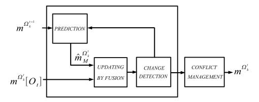
Figure 3: The Temporal Evidential Filter principle.
