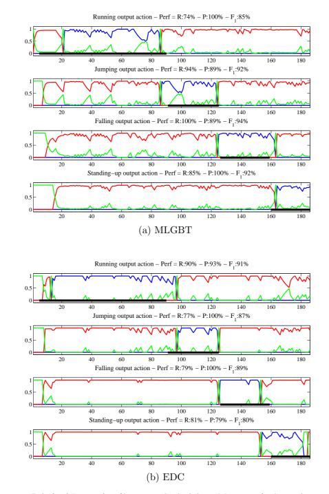
Figure 10: Beliefs of Fig. 9 after filtering and scheduling. Meaning of color is the same as in Fig. 9. Note that the beliefs on  $T_k^t$  (action  $A_k$  is true) are generally well detected when compared with the ground truth (bold black lines on the time axis).
