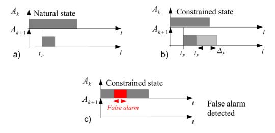
Figure 6: False alarm processing. a) Natural states of  $A_k$  and  $A_{k+1}$ . b)  $A_{k+1}$  is forced to be in a *true* state. c)  $A_{k+2}$  does not become true and the quality of  $A_{k+1}$  is bad, thus  $A_{k+1}$  is forced to be *false*.
