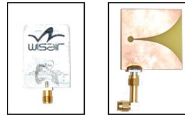
Figure 8. Antennas used on the wisair kits. (a) quasi-omnidirectional Wisair antenna (b) high gain Vivaldi antenna
