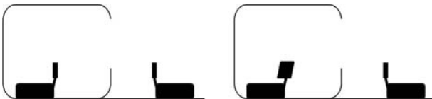
Figure 13. The orientation of antennas has no impact on the received power level as the cavity is homogeneous and pseudo-isotropic.
