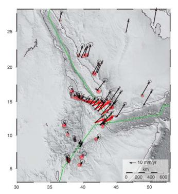
**Figure 1.** Map of the Nubia–Arabia–Somalia plate boundary region showing GPS-derived velocities with respect to Eurasia and 95% confidence ellipses (black arrows). Red arrows show residual velocities from a block rotation model for the Nubian, Arabian, and Somalian plates. Relative Euler vectors for the rotation parameters are given in Table 1. Topography and bathymetry from SRTM30 PLUS (see http://topex.ucsd.edu/WWW\_html/srtm30\_plus.html). Plate boundaries are shown schematically.
