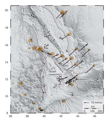
**Figure 2.** Map of the Afar Triple Junction showing GPS velocities and 95% confidence ellipses with respect to Nubia (see Table 1 for rotation parameters). Focal mechanisms (lower hemisphere projections) from Harvard catalog, 1976–2009. Topography and bathymetry as in Figure 1.
