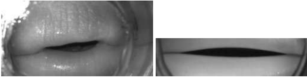
Figure 7: Maximum width of the opening of the lips of ( left ) player TJ playing the note Bb_2 at mf and ( right ) the artificial mouth playing note E_3 at 97dB
