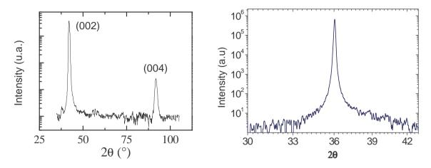
Figure 3: X-Ray diffraction diagram of an AlN thin film.
