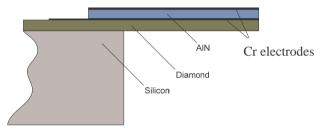
Figure 1: Schematic of a nano-crystalline diamond cantilever with piezoelectric AlN thin film..
