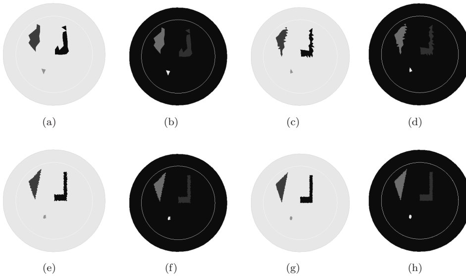
Figure 5. Reconstruction tests for different “imperfect” meshes: (a) \gamma and (b) q using a regular mesh with 50 boundary points, (c) \gamma and (d) q using a regular mesh with 100 boundary points, (e) \gamma and (f) q using a regular mesh with 200 boundary points and (g) \gamma and (h) q using a regular mesh with 400 boundary points.
