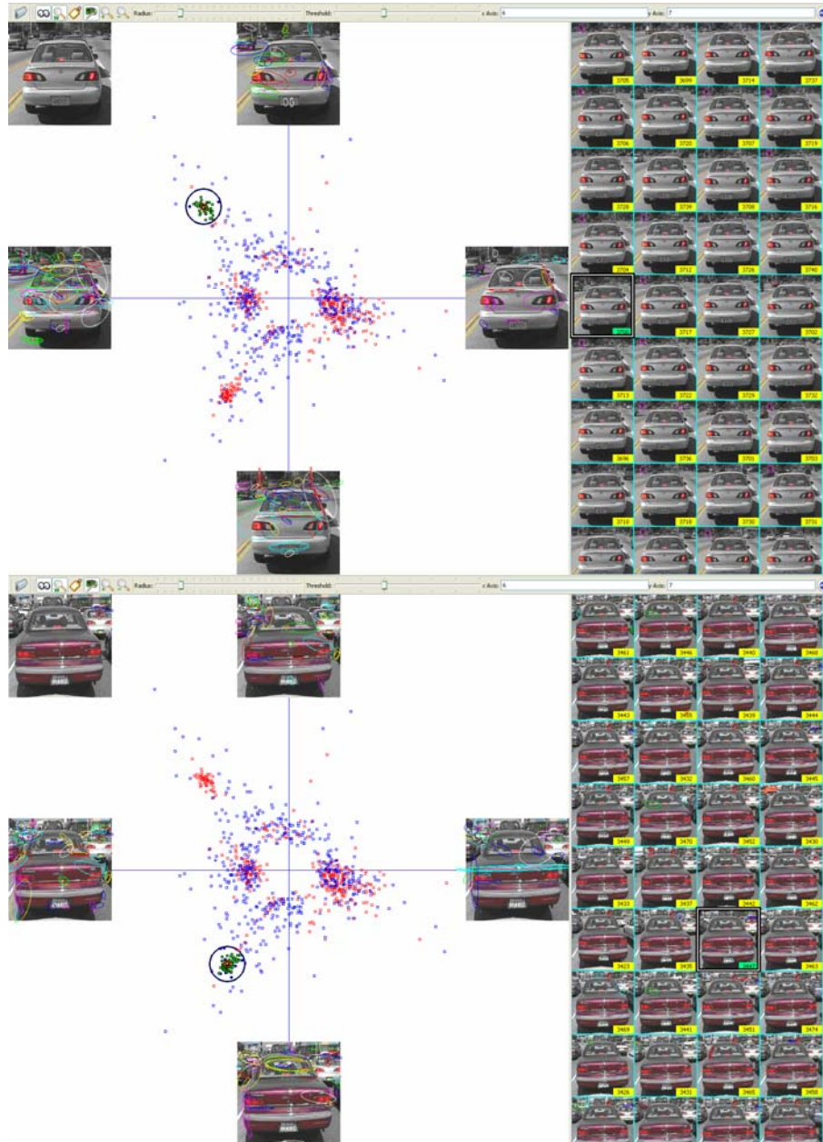
Figure 11. Topic discovery by projecting points on the best plane: we found two different topics “cars” on the plane 6 – 7
