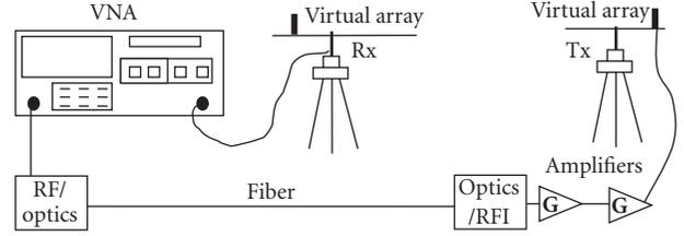
FIGURE 2: Principle of the channel sounder setup.
