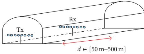
FIGURE 3: Configuration of the wideband MIMO measurements.
