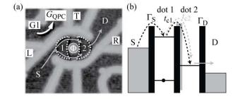
FIG. 5: (a) Scanning force microscope image of the double quantum dot with integrated charge read-out used for the self-interference experiment. (b) Schematic energy diagram of the double quantum dot system in the situation in which interference can be observed. The dashed arrows indicate the cotunneling-in process. Black and gray dashed arrows indicate the two alternative paths that enclose a magnetic flux  $\Phi = BA$  used to tune their relative phase.
