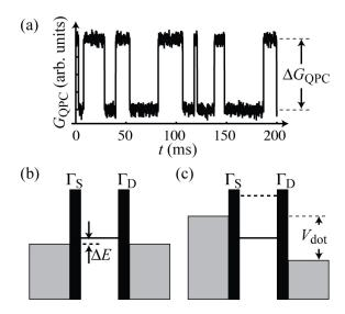
FIG. 2: (a) Time resolved signal of a quantum point contact detector measured close to a conductance resonance of the quantum dot. The signal switches randomly by  $\Delta G_{\rm QPC}$  between two distinct levels. (b) Schematic energy diagram of the quantum dot showing the situation  $V_{\rm dot} = 0$ . (c) The same for  $V_{\rm dot} \gg k_{\rm B}T$ .
