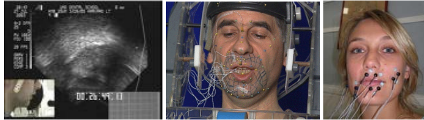
Figure 3. Capturing signatures of speech-production. Left-to-right: ultrasound imaging (from (Hueber, Chollet, Denby, Dreyfus, & Stone, 2007)), electromagnetoarticulography (EMA), electromyography (EMG).
