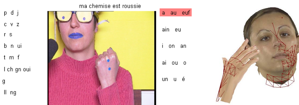
Figure 5. Cued speech processing. Left: impressive recognition scores (Aboutabit et al., 2007) are obtained by fusing lip and hand movements. Motion capture is simplified here by make-up. Right: text-to-cued speech synthesis (Gibert et al., 2005) is performed by concatenating elementary gestural units gathered by motion capture on a human speech cuer.
