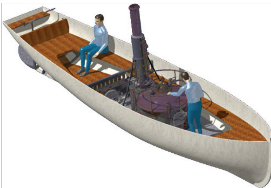
Figure 7. Digital Mock-Up of the steam boat of 1861
