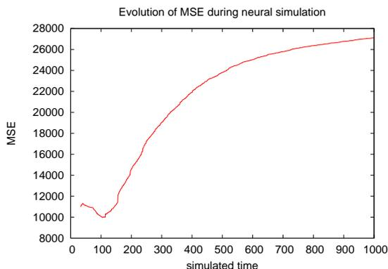
Figure 3: The MSE is computed for each time step during a neural simulation (here for Gaussian noise with  $\sigma = 85$ ). These data are processed to determine the “worst” and “best” values for neural filtering.
