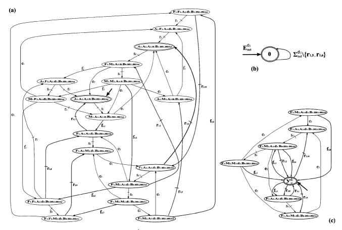
Fig. 7. Manufacturing system example: (a) the new model  $H_{\text{lab}}^{d_1}$  (extended controlled process of degraded mode  $d_1$ ) including the new model  $E^{d_1}$  (modified intermodal specifications); (b) the model  $E_{\text{out}}^{d_1}$  (switch Specification) to forbid undesired commutations  $r_{1,5}$ ,  $r_{1,6}$ ; and (c) the merged model  $H_{\text{merge}}^{d_1}$ , of degraded mode  $d_1$ , representing the final control law for this mode.
