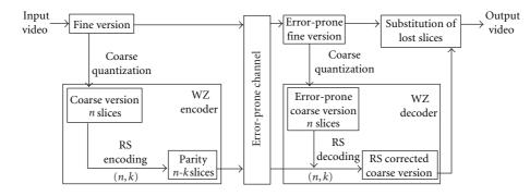
FIGURE 1: Block diagram of the SLEP scheme proposed in [4].
