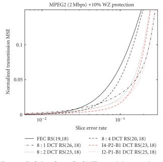
FIGURE 5: Evolution of normalized MSE transmission correction as a function of the incoming slice error rate.
