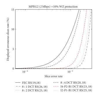
FIGURE 4: Evolution of the displayed erroneous slices rate after RS correction as a function of the incoming slice error rate.
