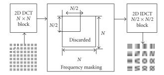
FIGURE 3: Spatial resolution downsizing by frequency filtering.
