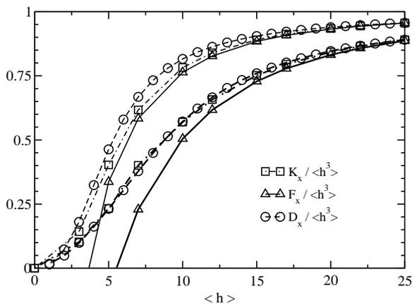
Figure 3: Normalized permeabilities of a rough fracture for flow normal to  $\vec{\lambda}$  as function of the fracture opening  $\langle h \rangle$  for two lateral displacements (Thick solid lines  $\vec{\lambda} = 10\vec{e}_y$  - Solid lines  $\vec{\lambda} = 20\vec{e}_y$ ). Despite the flow direction, the conditions are similar to the ones of Fig. 2 and circles, squares and triangles referred to  $D_x$ ,  $K_x$  and  $F_x$ .
