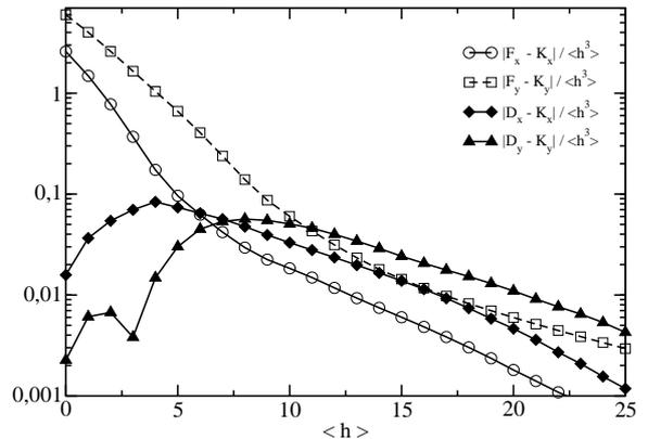
Figure 4: The relative errors  $|F_x - K_x| / \langle h^3 \rangle$ ,  $|F_y - K_y| / \langle h^3 \rangle$ ,  $|D_x - K_x| / \langle h^3 \rangle$ , and  $|D_y - K_y| / \langle h^3 \rangle$  as a function of the average fracture aperture  $\langle h \rangle$ . The data has been averaged over 10 samples, each of size  $512 \times 512$ , Hurst exponent  $H = 0.8$  and lateral displacement  $u = 10$ .
