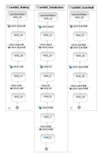
Figure 6. State machines for the AIBO object
