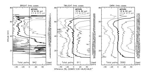
**Fig. 4.** Validation results for the different limb illumination conditions. Left panel: bright limb; middle panel: twilight limb; right panel: dark limb cases. All plots show the median difference (thick black line) between GOMOS and the validation data together with the 16 and 84 percentiles (thin dark grey lines) and the 2.5 and 97.5 percentiles (thin light grey lines). On the right side of each panel is the number of collocated pairs used for the corresponding altitude.
