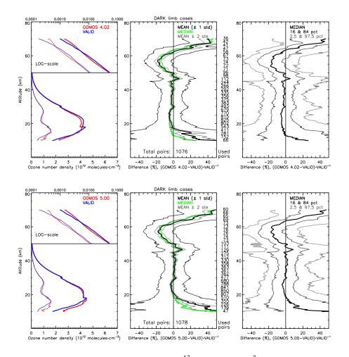
Fig. 2. As Fig. 1, except filtered for ozone values below 0 and above  $10^{13}$  molecules per cm<sup>3</sup> and with some Thule, Dumont d'Urville and Legionowo collocations removed.
