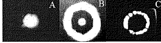
FIG. 12. Sample photographs of the fiber output end showing distribution of energy between the two cores at different wavelengths: (A) light in the central core only at 633 nm, (B) light distributed over the two cores as the supermode at 1550 nm, (C) light in the external core only at 633 nm.
