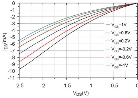
FIG. 2. (Color online) Measured dc  $I_{DS}$  vs  $V_{DS}$  at different  $V_{GS}$ .
