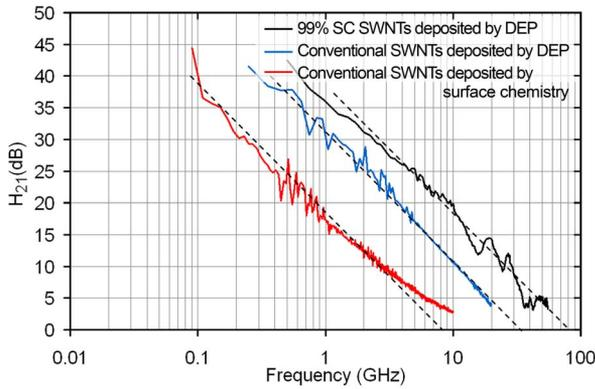
FIG. 5. (Color online) Current gain  $10 \log_{10}(|H_{21}|^2)$ , extracted from the  $S$  parameters for the three SWNT FET cases. The dashed lines correspond to the ideal slopes of  $-20$  dB/decade for  $|H_{21}|$ . The respective  $f_c$  are: 8 GHz, 30 GHz and 80 GHz.
