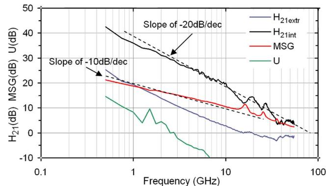
FIG. 4. (Color online) Current gain  $10 \log_{10}(|H_{21}|^2)$ , MSG,  $U$  (in decibels), extracted from the  $S$  parameters. The dashed lines correspond to the ideal slopes of  $-20$  dB/decade for  $|H_{21}|$  and  $-10$  dB/decade for MSG.
