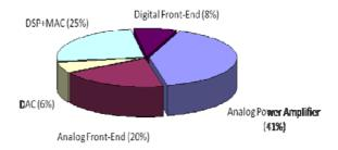
Figure 6 : OFDM transmitter power consumption budget
