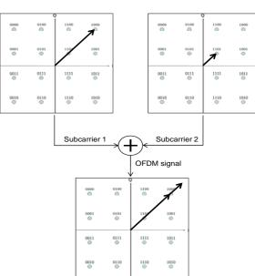
Figure 7 : The power of the OFDM signal could be the sum of the maximum power of each subcarrier.
