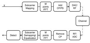
Figure 5 : OFDM transceiver structure
