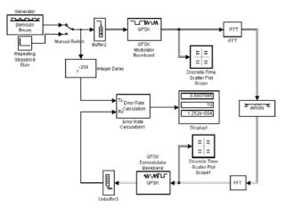
Figure 11 : Simple Simulink model for OFDM transceiver
