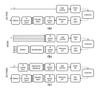
Figure 8 : Transmitter structures of SC/FDE (a), OFDM (b) and SC-FDMA (c)
