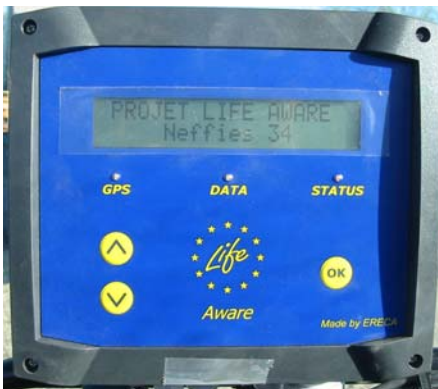
Fig 1: The MPU unit in the tractor cabin
