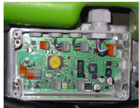
Fig 2: the APU box on the sprayer.
