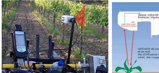
Figure 8: Capteur Greenseeker, installation (source [http:// www.ntechindustries.com](http://www.ntechindustries.com))
