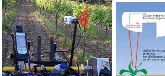
Figure 8: Capteur Greenseeker, installation (source http:// www.ntechindustries.com )
