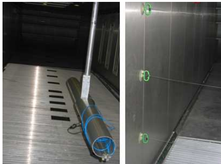
Figure 2. Installation of the collectors in wind tunnel; left: Carpets on the ground, (under the boom) - right: PVC lines
