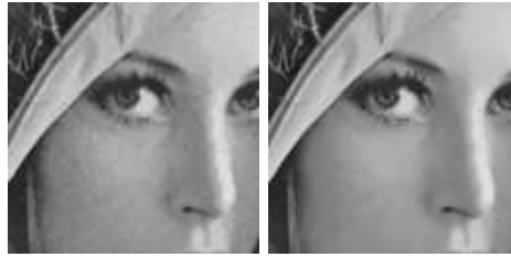
FIG. 3.7. Left and right: extract of the result of the NLmeans filter with s^2 = 3 \times 3 and s^2 = 5 \times 5 on a noisy image ( \sigma = 10 , h optimized for PSNR). Using a too small patch size makes the algorithm less robust to noise and Lena's skin looks mottled. It looks smoother with patch size 5 \times 5 but visual artifacts appear in the eye.
