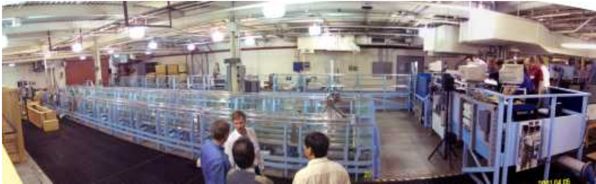
Figure 6. Model canal in Reclamation's Hydraulics Laboratory
