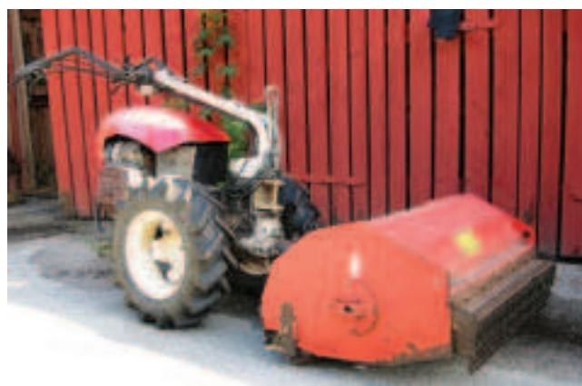
◊ Denmark Photo 2.3 | Two-wheeled tractor with flail mower attachment, used for mechanical vegetation management in forests owned by the municipality of Vejle, where herbicide use since 2003 is prohibited through a voluntary agreement.
