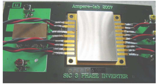
Fig. 13. Latest prototype. A 540VDC 15A three phase inverter operating at 200°C
