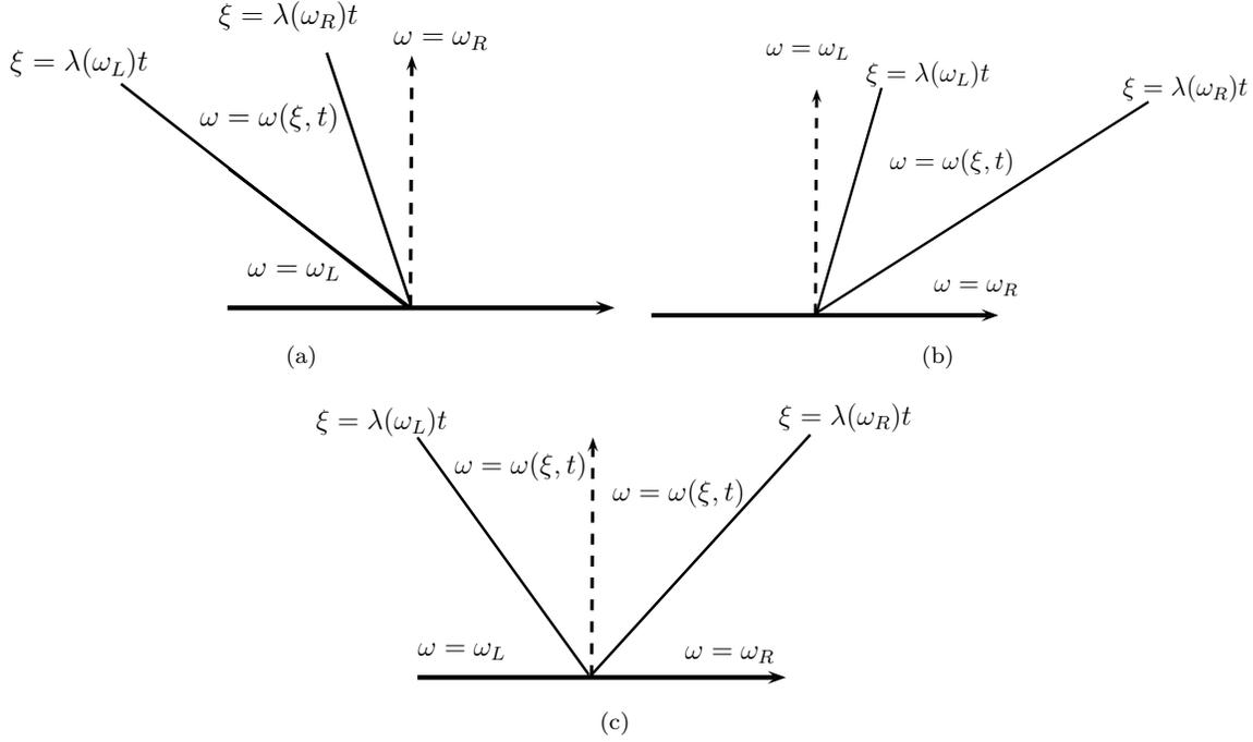
Figure 5: Rarefaction situations with  $\omega_0 \neq 0$ . Three cases arise in function of  $\omega_L$  and  $\omega_R$  signs:  $\omega_R > 0$  (a),  $0 > \omega_L$  (b),  $\omega_L > 0 > \omega_R$  (c).
