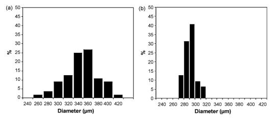
Fig. 8. Typical size distribution of particles diameters obtained in (a) the threshold zone and (b) the decreasing zone. CVs are equal to 9% (a) and 3% (b).
