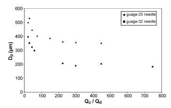
Fig. 4. Average diameter of polymer particles produced with two different needles (viscosity of the continuous phase is equal to 500 cP).
