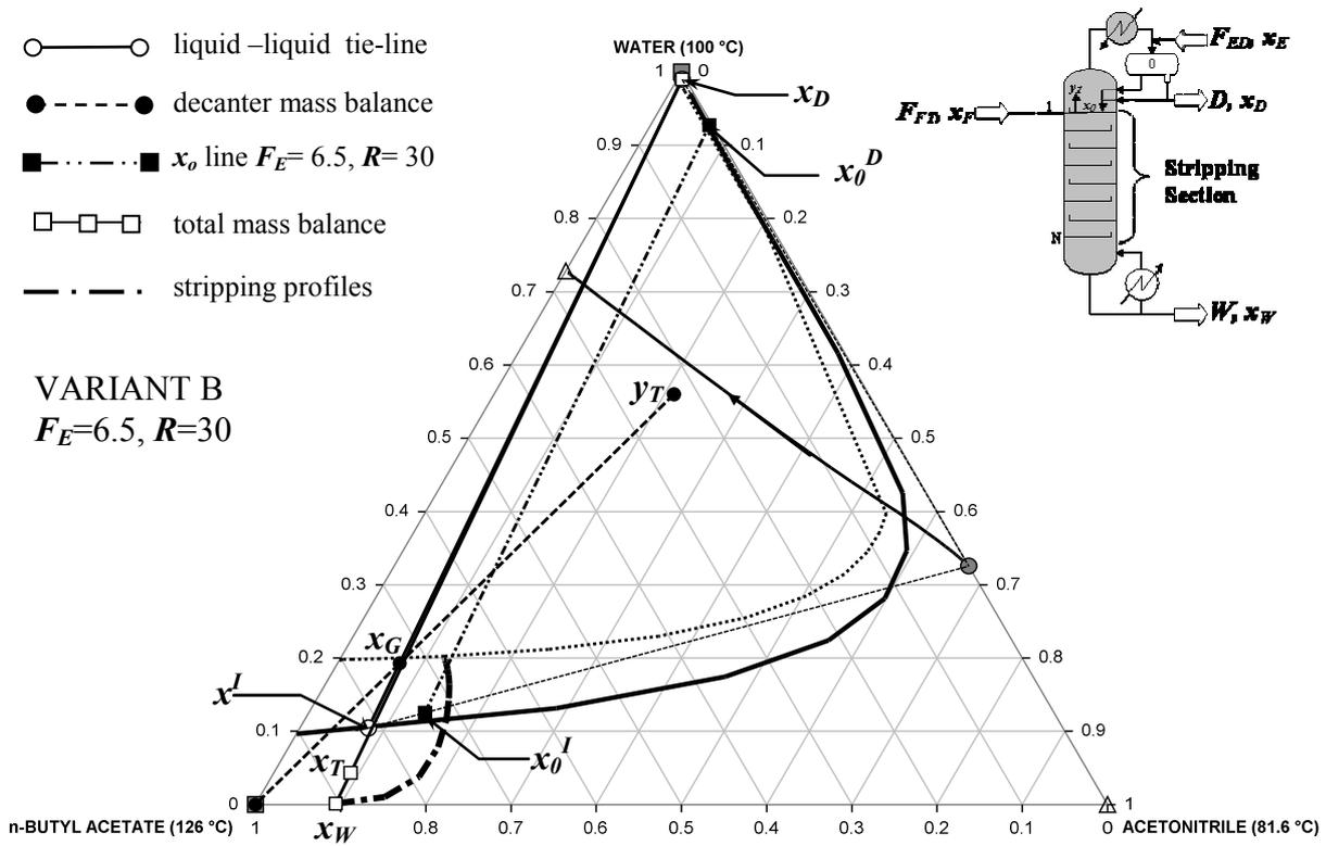
**Figure 12. Stripping composition profile for column configuration 7 considering two operating conditions: Variant A ( $F_E=2, R=10$ ) and Variant B ( $F_E=6.5, R=30$ ).**
