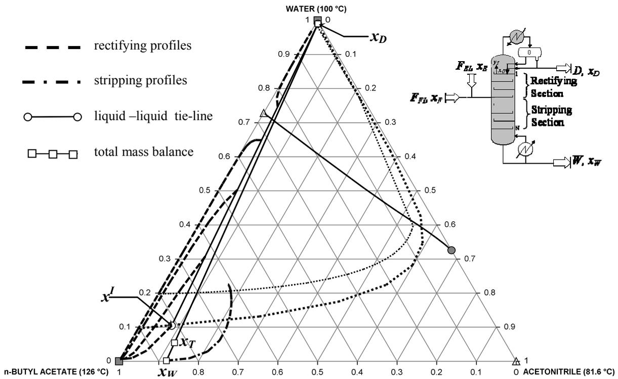
**Figure 5.** Map of rectifying composition profiles computed from several  $x_R$  points, and the stripping composition profile computed from  $x_W$ , for the heterogeneous continuous distillation (configuration 1).
