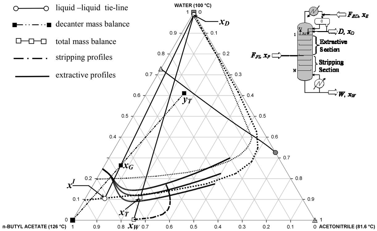
**Figure 10. Stripping liquid composition profile and map of extractive composition profiles for feeding the entrainer recycled stream into the decanter, and the main azeotropic feed at an intermediate point of the column (configuration 5).**
