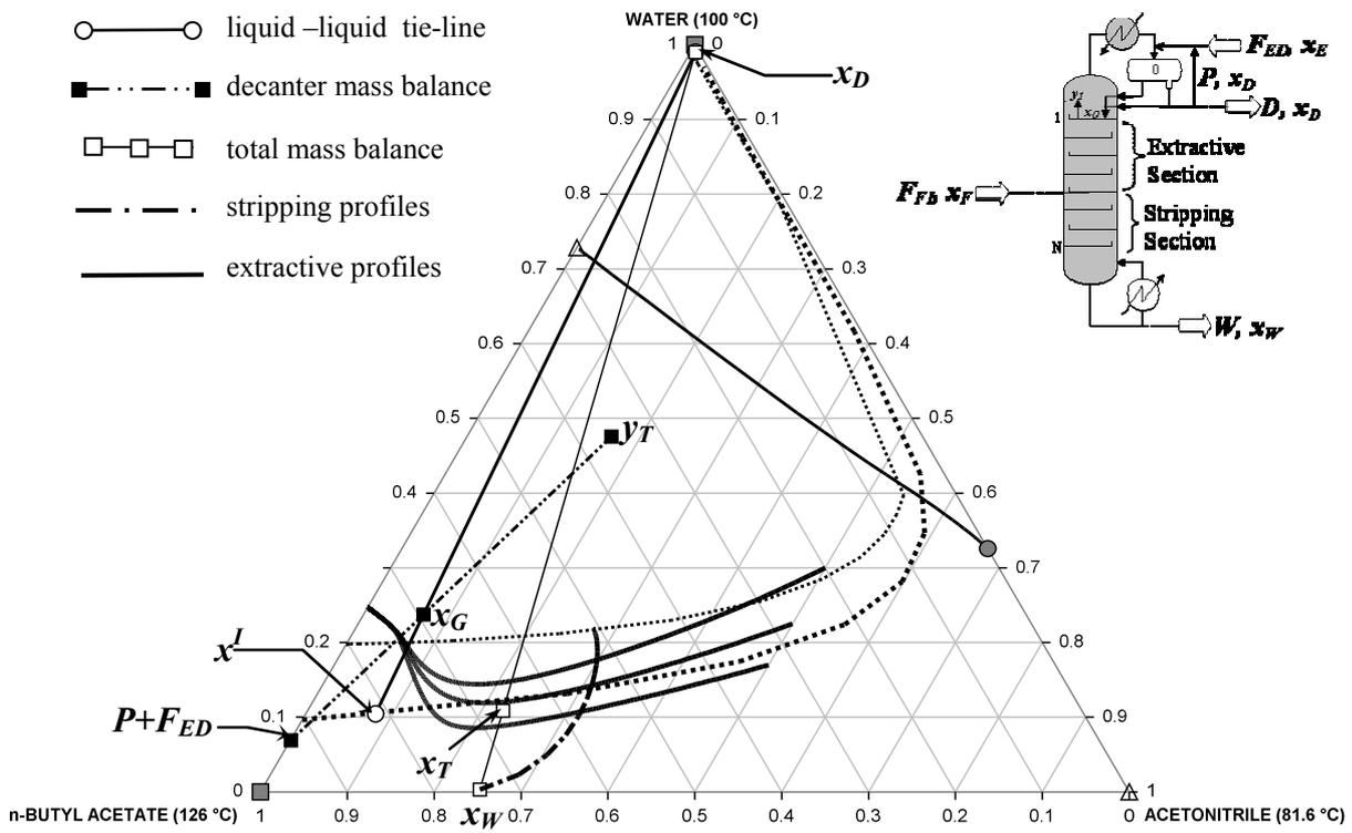
**Figure 11. Stripping and extractive composition profiles when the main azeotropic stream is fed at intermediate point of the column, and both the entrainer recycle stream and a portion of distillate are sent to the decanter (configuration 6).**
