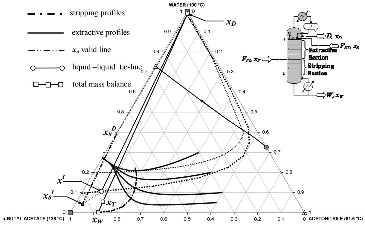
Figure 7. Stripping liquid composition profile and map of extractive composition profiles for heterogeneous distillation (configuration 3).
