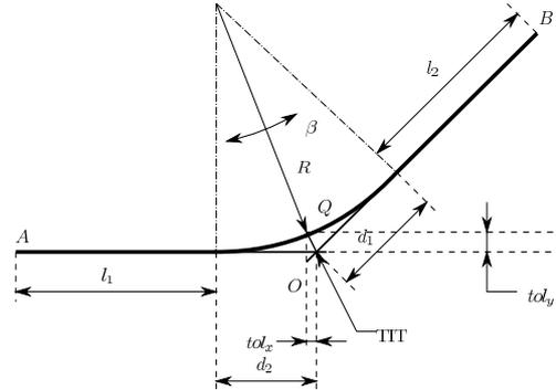
In the literature, a circle arc is used to model this transition [14]. Radius  $R$  of this circle arc is calculated in relation to the tolerance permitted by the NC and lengths  $l_1$  and  $l_2$  of the blocks before and after the discontinuity:
