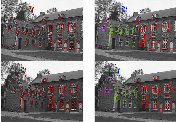
(b) A unique group is detected when using epipolar geometry (c) 4 groups are detected with homography
