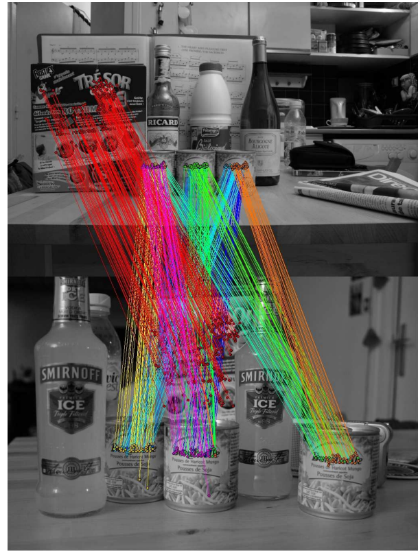
(b) The MAC-RANSAC algorithm is able to detect the 10 different groups of correspondences.
