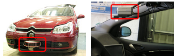
Fig. 7. Experimental platform: Lidar (left), Camera (right)
