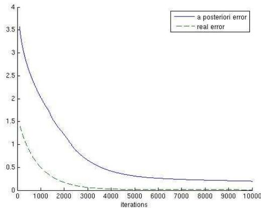
Figure 4: Comparison of the relative  $L^2$  error with the predicted *a posteriori* bound.
