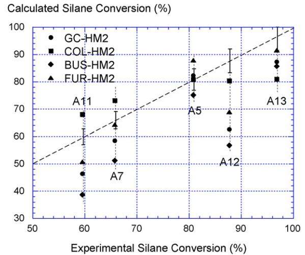
Fig. 7. Calculated silane conversions vs. experimental silane conversions.
