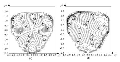
Figure -6. Isoconditioning loci of the matrix (a)  $\overline{\bf A}_1$  and (b)  $\overline{\bf A}_2$  with R/r=2 and l/r=2
