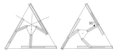
Figure -2. Parallel singularity
