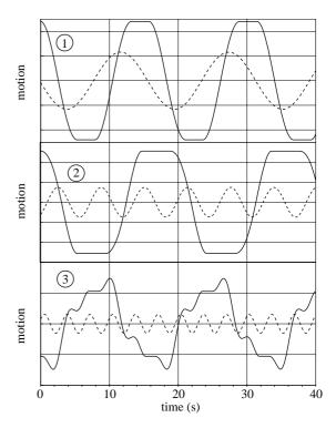
Fig. 4. Numerical simulations of the motion of a mechanical oscillator with and without latching control (alternated maxima ramps);  $\omega_0$ =0.6,  $\mu$ =0.1,  $F_{\rm ex}$ =1,  $\omega$ =1.
