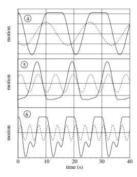
Fig. 7. Numerical simulations of the motion of a mechanical oscillator with and without latching control (equal ending ramps);  $\omega_0$ =0.6,  $\mu$ =0.1,  $F_{\rm ex}$ =1,  $\omega$ =1.
