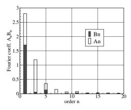
Fig. 6. Fourier coefficients of the velocity  $\dot{\zeta}$  of the controlled motion of Fig. 4b.
