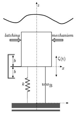
Fig. 1. A generic single DoF wave energy device.
