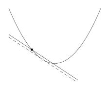
Considering integrality constraints make problems more complex to solve. In particular, the optimality conditions do not hold at local optima.
