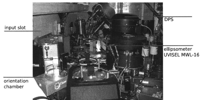
FIG. 1. Overview of the platform DPS CENTURA 5200 from Applied Materials with in situ spectroscopic phase-modulated multiwavelength ellipsometer UVISEL MWL-16 from Horiba Jobin Yvon.
